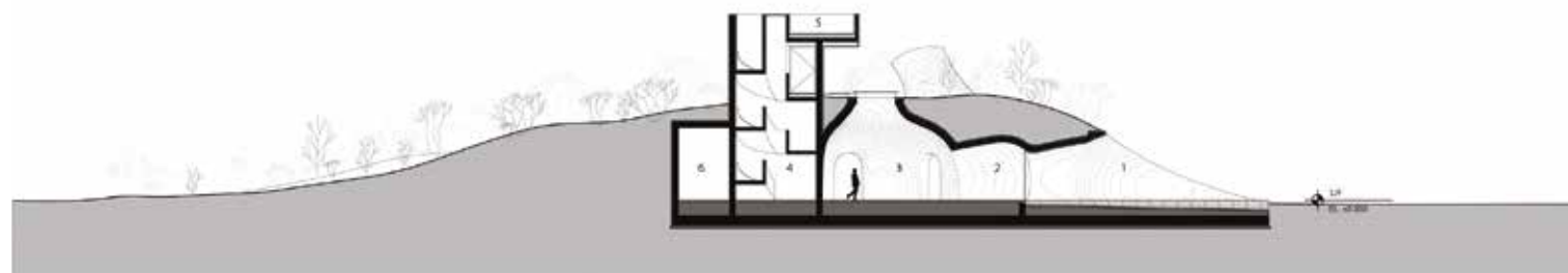
Section A1 Outdoor Exhibition Terrace 2. Secondary Entrance 3. Gallery 4. Stairs 5. Viewing Platform 6. Toilet
